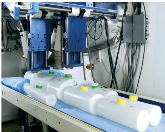
Figure 1 A whole-body radiation monitor
